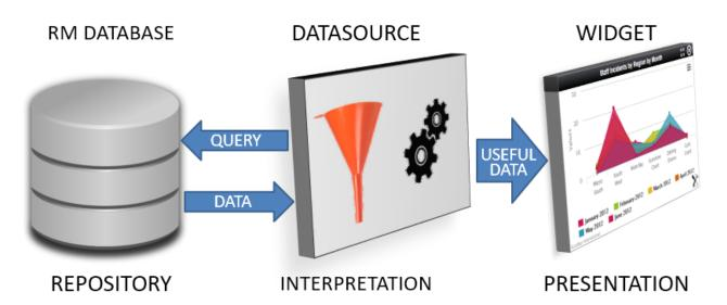
A Datasource contains the background properties which can then in turn be displayed as a widget. The Datasource contains all the configuration information such as the type of chart used, the register the information will be extracted from (incidents, feedback etc.), and any specific filters applied (e.g. site, location, gender etc.)Once this Datasource has been built, it can be shared with **C**RLDatix
