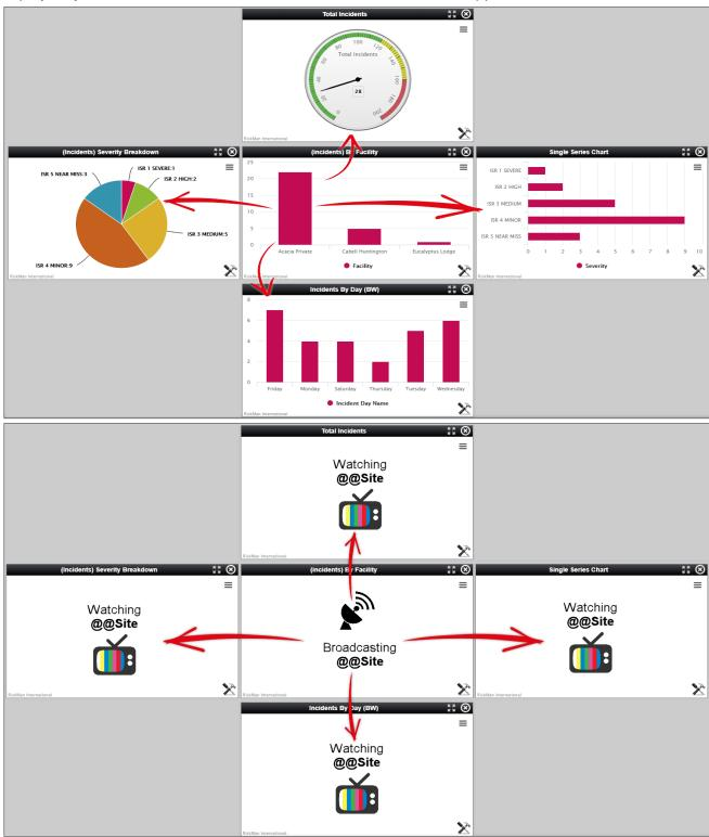
The example above shows one central Widget changing the data displayed in the four surrounding Widgets. The Watching Widgets will display only data for the Location that was selected in the Broadcasting Widget.
